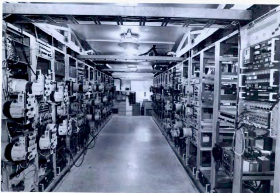
Interior of a diagnostics recording station with oscilloscopes and cameras.
